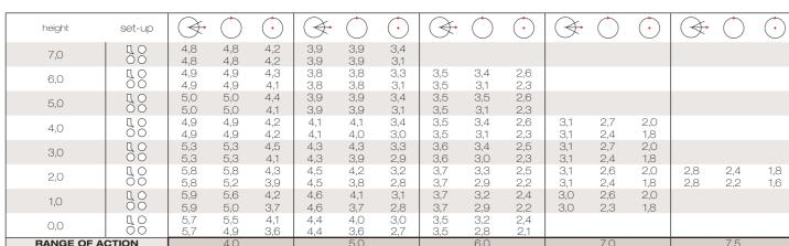
• The values, indicated in tons, are to be considered as: at hook, with no lifting device applied; with machine idle, on a flat and horizontal surface, not soft, and with oscillating axle blocked.
