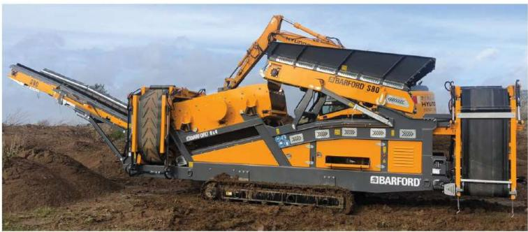
Barford S80 Scalper Screen 8'x 4' Double Deck with 180° Radial Fines Conveyor, Powered by a CAT 3.4 Engine, Feeder Belt Width 1000mm, Fine Conveyor Belt Width 800mm, Mid Conveyor Belt Width 650mm, Transfer Conveyor Belt Width 1000mm, Oversize Conveyor Belt Width 1050mm. Hyd Adjustment to Change from Three Way to Two Way Split.
