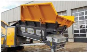
Cat 4.4 Accert 96kw Engine, Tracked Low Level Conveyor 80ft x 48", Twin Gearbox Drive, Twin Drive Discharge Belt, Cast Iron Pumps, Hyd Slew Hubs, Hyd Legs Under Feeder, Hyd Fold on Discharge, Galvanized Legs & Check Valves in Rams, 18m³ Hopper Capacity.
